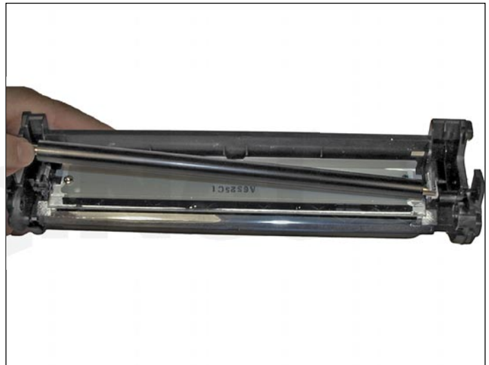
12. Clean the two PCR holders and place a small amount of conductive grease on the black PCR holder. Install the PCR.
