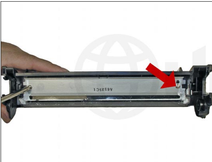
11. Lightly coat the new blade with your preferred lubricant.
